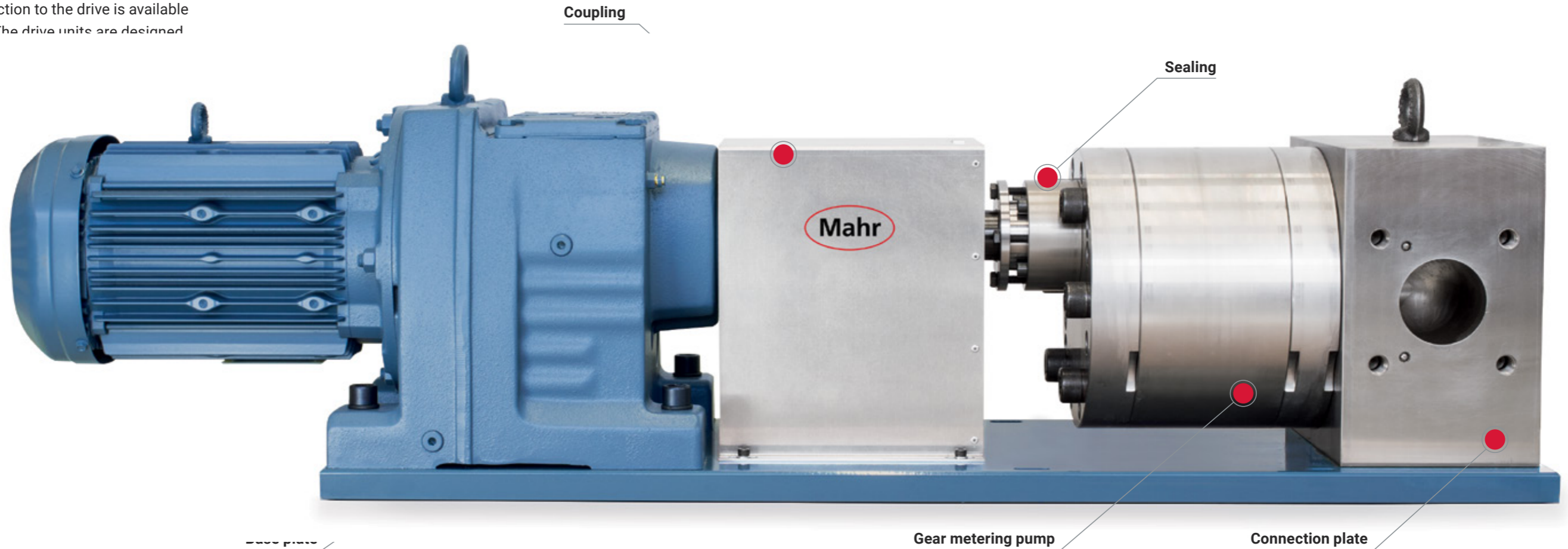
Drive unit with gear metering pump type 300 cc / rev.
